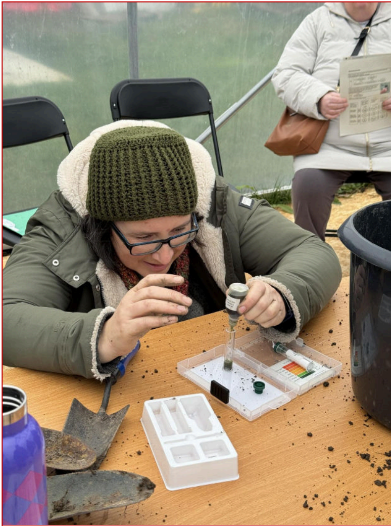
Lucy demonstrates how a sample of soil can be added to the testing solution.
